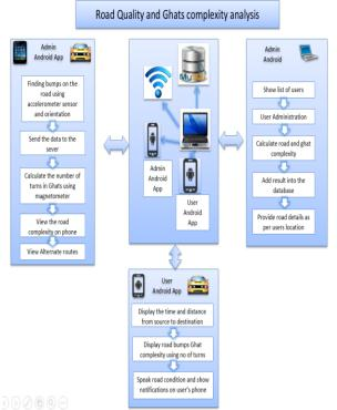
Fig.1 Conceptual image of continuous road condition monitoring system
